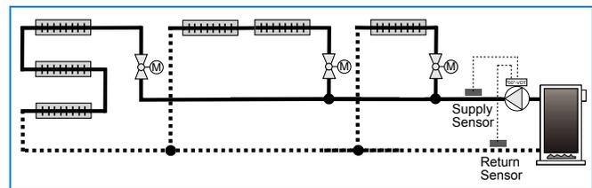
The solution? The Taco 00-VDT circulator will automatically adjust its speed to maintain the designed for 20° delta T across the open zones. The circulator will speed up or slow down as needed, as zones open or close, always maintaining a 20° delta T. This will increase overall comfort and sharply reduce boiler short-cycling. The 00-VDT will also control velocity noise issues in the system, eliminating the need for a pressure differential bypass valve.
